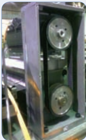
Press feed machine built with a conventional servomotor, gearhead, belt and pulleys.
