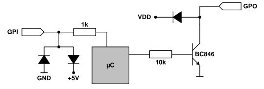
Figure 4.6: Wiring scheme for GPO and GPI
