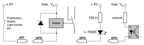
Figure 4.7: Examples for possible wirings for GPI and GPO
