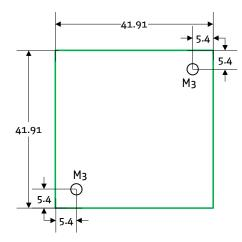
Figure 4.1: Board dimensions and mounting holes (all dimensions in millimeters)
