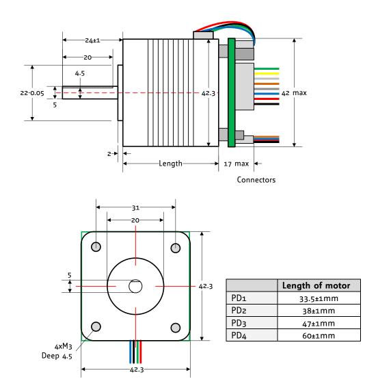
Figure 4.2: Dimensions of the PDx-110-42
